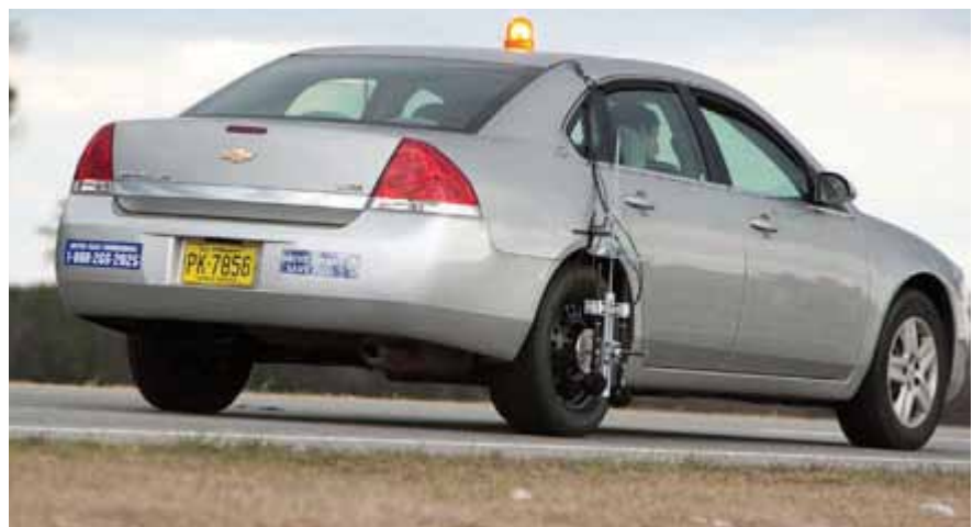
Data collection equipment measures pavement noise while a vehicle travels down the highway.
