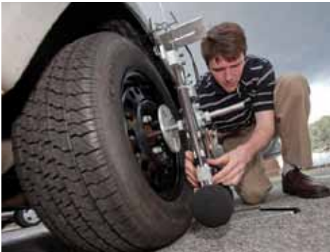
ECU graduate Richard Shores prepares a noise meter for a road test. Shores assisted in the highway noise research while a graduate student at ECU. (Photos by Cliff Hollis)
